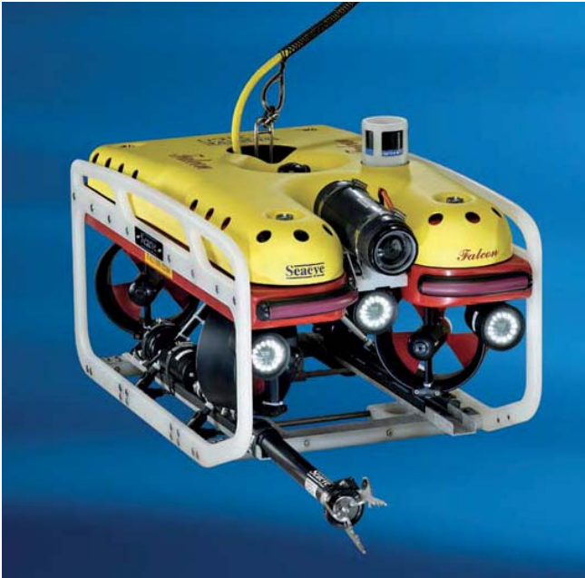
© SAAB Seaeeye - Falcon with single function, 3 jaw manipulator
