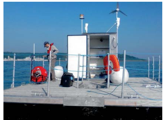
© DGA / RTSys / ISEN / Marée - MIMO underwater acoustic communication experiment, Sea Test Base, Lanvéoc
