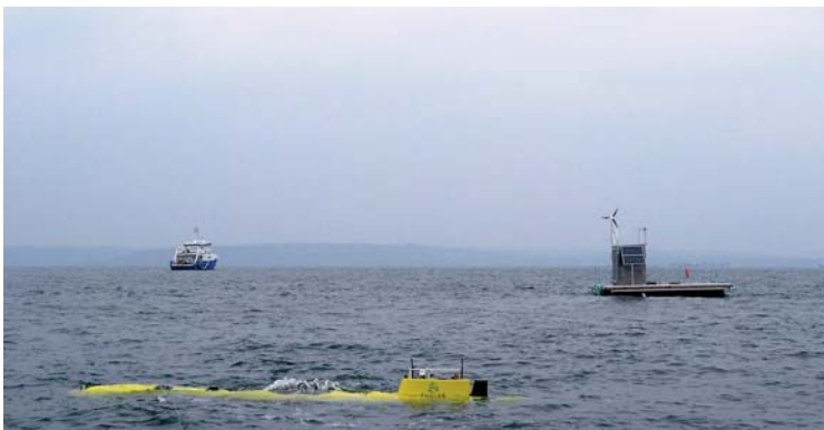
© Thales / ECA Robotics, AUV remote monitoring from the shore via the instrumented pontoon (radio link and underwater acoustic communication), Sea Test Base, Lanvéoc
