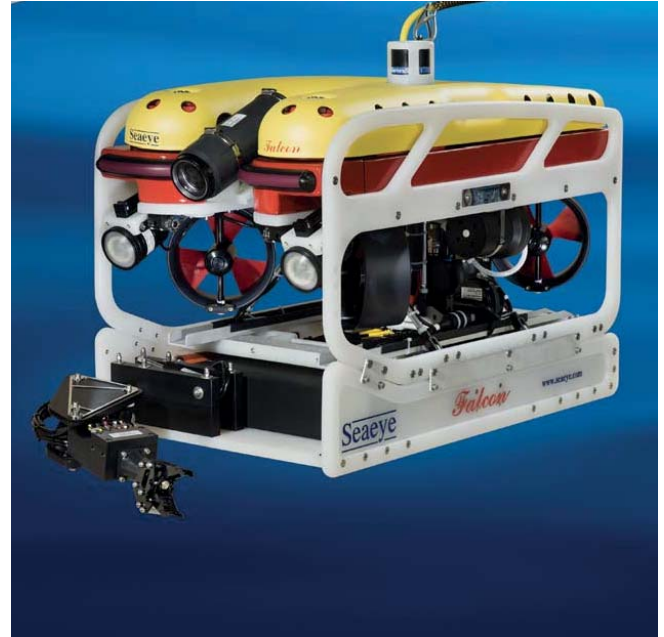
© SAAB Seaeeye - Falcon DR with 5 function manipulator
